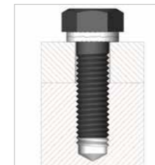
Hexagon bolt secured in a blind hole
