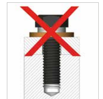
No locking function when combined with flat and freely rotating washers
