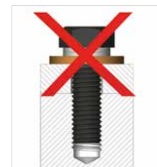
No locking function when combined with flat and freely rotating washers
